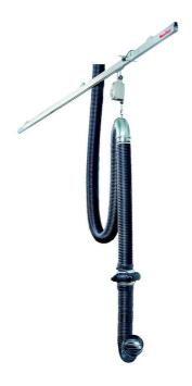
MagnaTrack ST is designed for stations with fewer runs. The free-hanging exhaust hose is equipped with a swivel attached to a balancer, which moves on the guide track. A switch on the track separates the entire hose assembly from the vehicle in a one-step process, minimizing stress or strain from the vehicle to the exhaust hose or ceiling brackets. MagnaTrack ST is available in lengths from 6 to 12 m (20 to 40 ft) and it fits vehicles with low mounted exhaust pipes.
