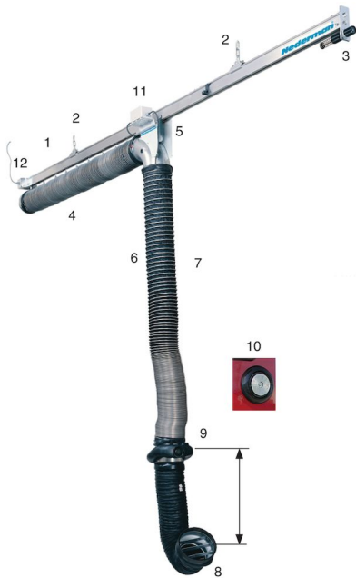
1. Track, 2. Bracket, 3. Rubber stop, 4. Horizontal exhaust hose, 5. Trolley, 6. Elastic cord, 7. Vertical exhaust hose, 8. Nozzle, 9. Electro-magnet assembly, 10. Anchor plate, 11. Disconnection box, 12. Transformer
