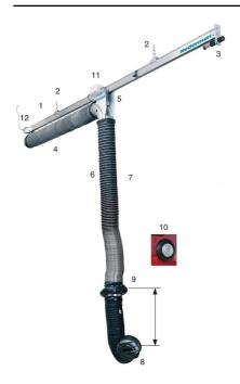
The MagnaTrack S is an economical alternative to MagnaTrack HS designed for a normal frequency of runs and exit speeds. Magnatrack S has an elastic cord inside the exhaust hose (instead of a balancer) and a rubber stop (instead of a hydraulic trolley stop). The track system serves one vehicle at a time. MagnaTrack S is available in lengths from 3.5 m to 18 m; (10 ft. to 60 ft.) and it fits vehicles with low mounted exhaust pipes.
