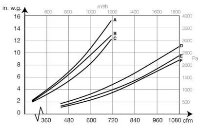
X: airflow m3/h Y: static pressure Pa A= 4 m Ø125 mm, B= 3 m Ø125 mm, C= 2 m
