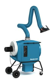
The FilterBox 12A is equipped with a powerful fan for a maximum air flow capacity of 1 200 m3/h (700 CFM). An integrated silencer reduces noise from the fan and outlet air. The unit has an advanced filter control system with automatic cleaning that starts when the air flow is too low. Available either as a mobile unit on wheels or attached to a floor stand. Additional protection from harmful particles is provided if a HEPA filter is installed.
