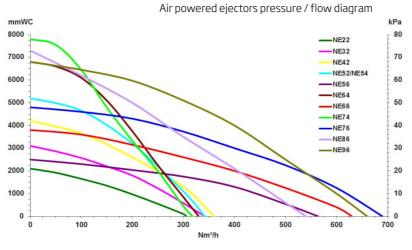
Air Powered ejectors
