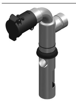
Handy pre-separator for liquids for collection into oil drums. It should be placed in the bung hole (R2") of an empty but suitable oil drum. By connecting the unit to suction hoses, it is ready to use. The built-in float ball stops the suction when the drum is full.
