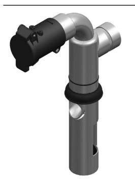
Handy pre-separator for liquids for collection into oil drums. It should be placed in the bung hole (R2") of an empty but suitable oil drum. By connecting the unit to suction hoses, it is ready to use. The built-in float ball stops the suction when the drum is full.
