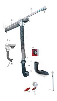
The MagnaTrack HS is designed to serve emergency stations with a high frequency of runs. The track system serves one vehicle at a time. The balancer has a constant liftning power. MagnaTrack HS is available in lengths from 3.5 m to 18 m; (10 ft to 60 ft) and it fits vehicles with low as well as high mounted exhaust pipes. Capacity: 1 vehicle per system
