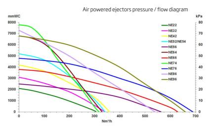
Air Powered ejectors
