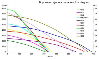
Air Powered ejectors
