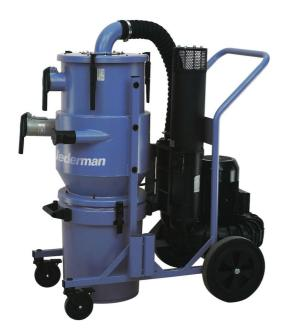
Very powerful electric powered industrial dry vacuum cleaner suitable for general cleaning, extraction of dust from grinding machines and for powder transportation. Filter cartridge category M as standard main filter and control filter. Filters are also available in HEPA/Absolute or washable polyester version. Efficient filter cleaning by manual reverse air jet. Thermal overload fitted as standard. With 50.8 mm and 76.2 mm(2in and 3 in); hose connections supplied on standard version
