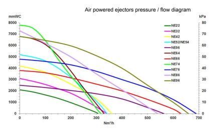
Air Powered ejectors
