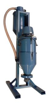
An extremely powerful vacuum unit for the collection of blasting grit and other granulated material. The combination of high vacuum and high airflow make material transport over long distance possible. Compact design, built on a frame with the possibility of transportation by forklift. Equipped with grit and dust separator. The clean grit is collected in a silo and can be re-used. The dust is trapped in a high efficient NCF filter and discharged into a dustbin or bag.
