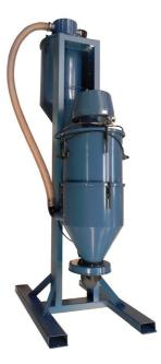
An extremely powerful vacuum unit for the collection of blasting grit and other granulated material. The combination of high vacuum and high airflow make material transport over long distance possible. Compact design, built on a frame with the possibility of transportation by forklift. Equipped with grit and dust separator. The clean grit is collected in a silo and can be re-used. The dust is trapped in a high efficient NCF filter and discharged into a dustbin or bag.
