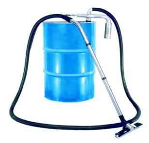
Handy ejector-driven drum filler for collection and transport of oil, chemicals, water and other liquids. It is placed in a bung-hole (R 2") of an empty but suitable oil drum. By connecting the unit to a compressed air hose and a suction hose, it is ready for use. Suction stops when the drum is full, due to the built-in float stop. The ejector is easy to mount on a variarity of drums. Drum is not included.
