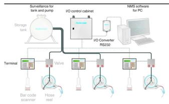
The NMS lubrication monitoring system for complete fluid control accurately monitors and supplies the correct amount of oils and liquids to each vehicle without manual handling or tapping. It also informs suppliers when it is time to refill tanks. This is the end of spillage, loss and unnecessary stoppages.
