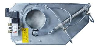
The TAV 100 and TAV 150 valves are mainly used as shut-off valves in the main branches of the pipework system. Because the valves can be opened and closed automatically, the vacuum is always concentrated on the connections, extraction points or machines in operation at the time. This maximises the power of extraction, produces lower operating costs and minimizes the size of the vacuum unit.
