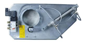
The TAV 100 and TAV 150 valves are mainly used as shut-off valves in the main branches of the pipework system. Because the valves can be opened and closed automatically, the vacuum is always concentrated on the connections, extraction points or machines in operation at the time. This maximises the power of extraction, produces lower operating costs and minimizes the size of the vacuum unit.
