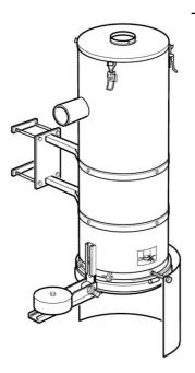
The KSA 70 has a cyclone inlet with an insert for the highest separation efficiency and wear protection. The outlet has a mechanical protection for over-filling, preventing material from being sucked into the pipework in large quantities. The balanced bottom lid opens downwards and is kept shut by the vacuum during normal operation. The installation normally requires a vacuum valve at the top of the separator, allowing emptying when the work station is not in use.
