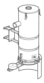
Pre-separation of metal chips and cutting fluids or similar materials near the work station to prevent wear on the pipe system.
