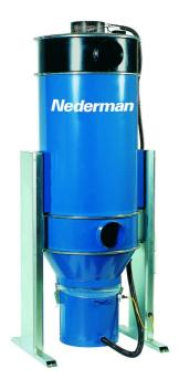
Dust collector with 2-stage filtration. Central inlet with velocity reducer. Fully automatic filter cleaning. Can easily be equipped with a great variety of filter materials, bins, emptying systems, etc. Standard equipped with circular bags of polypropylene. PTFE or antistatic filters on request.
