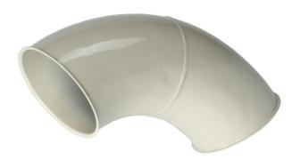
2 mm duct with clipped edge in steel quality SS 1312. Painted in RAL 7032 with Priming 50  $\mu$ m, zinc content 70%.
