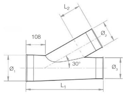
L1 =  $(02 \times 2) + 236$ L2 = (02/2) + 58Ø3 must be smaller than or equal to Ø1 Ø2 must be smaller than or equal to Ø3
