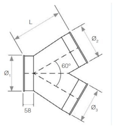
L = Ø1 + 100, Ø2 and Ø3 must be smaller than or equal to Ø1
