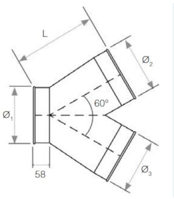
L = Ø1 + 100, Ø2 and Ø3 must be smaller than or equal to Ø1
