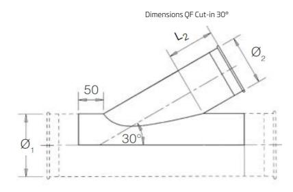
L2 =  $(\emptyset 2 / 2) + 58$ ,  $\emptyset 2$  must be smaller than or equal to  $\emptyset 1$
