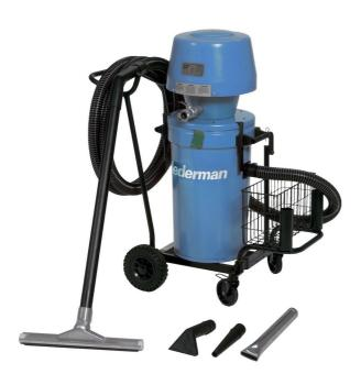
A high capacity vacuum unit for suction and transportation of various non-flammable liquids like oil, chemicals, mud, cooling liquids and water, as well as metal chips, sand, and other granules. The standard version vacuum unit can fill the container with liquids in a minute or two. Suction equipment is made for heavy duty work. The container is mounted to the trolley by brackets.
