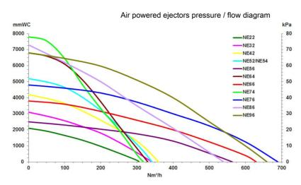
Air Powered ejectors
