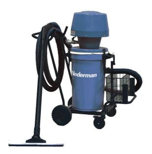
A high capacity vacuum unit for suction and transportation of various non-flammable liquids like oil, chemicals, mud, cooling liquids and water, as well as metal chips, sand, and other granules. The standard version vacuum unit can fill the container with liquids in a minute or two. Suction equipment is made for heavy duty work. The container can be tipped for ease of emptying.
