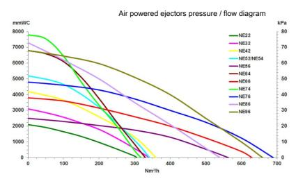
Air Powered ejectors
