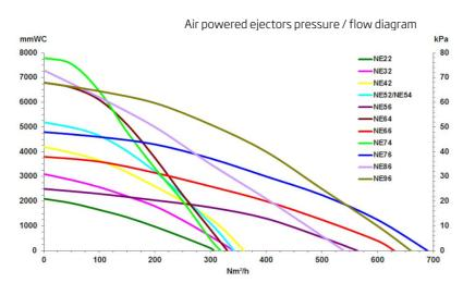
Air Powered ejectors
