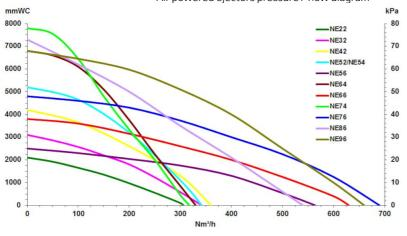
Air powered ejectors pressure / flow diagram
