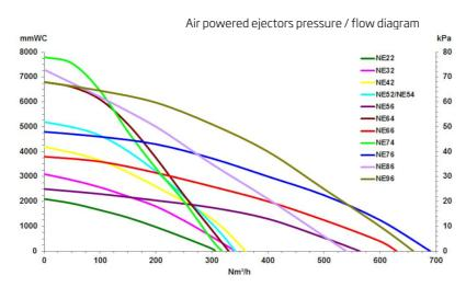
Air Powered ejectors
