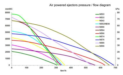
Air Powered ejectors
