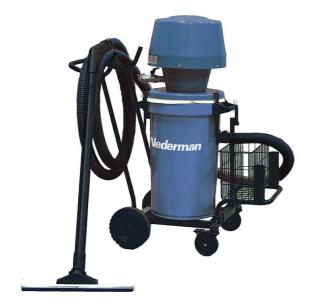
Wet/dry vacuum cleaner with a single container system for suction and transportation of various liquids like oil, chemical spillage, mud, cooling liquids, and water, as well as metal chips, sand, and other granules. The industrial vacuum cleaner can fill the container ith liquids in about a minute or two and the suction equipment is made for heavy duty work. The container can be tipped for ease of emptying.
