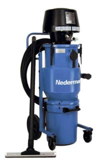
Fine dust problems are easily solved by this high capacity heavy duty industrial vacuum cleaner. Efficient cyclonic preseparation of the dust before the absolute/HEPA filter. A single container system with absolute/HEPA filter for collection of very fine dust and granulated material.
