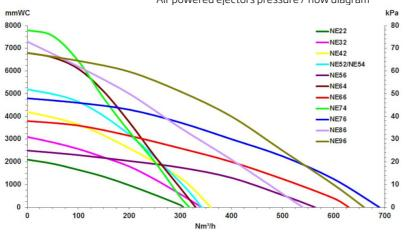
Air powered ejectors pressure / flow diagram
