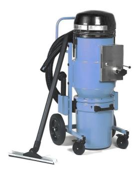
Fine dust problems are easily solved by this high capacity vacuum unit. Efficient cyclonic preseparation of the dust before the absolute/HEPA filter. Manual filter cleaning is easy and efficient. The single phase multistage fan system creates high airflow for excellent material collection and transportation. The unit may be equipped with a larger container.
