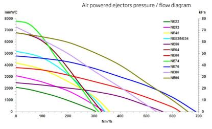
Air Powered ejectors
