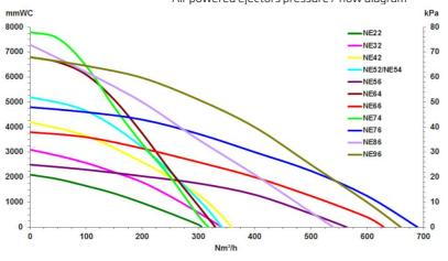
Air powered ejectors pressure / flow diagram
