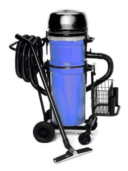
Electrical driven industrial vacuum cleaner, designed for extraction of dusts such as powder, granules and hazardous materials. By installing a disposable filter bag in the container the dust can be collected directly into the bag. Thereby contact with e.g. collected hazardous material is minimized. The dry vacuum cleaner equipment is light and easy to handle.
