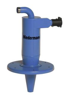
Cyclones are normally used when a maximum pre-separation of collected material from the transportation airflow is required. Cyclones are normally located on silos, tanks, containers etc. suitable to store the collected material and thereby function as a deead chamber under the cyclone. Normally, a filter stage shall be installed between the cyclone and the vacuum power unit.
