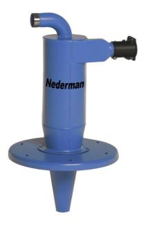
Cyclones are normally used when a maximum pre-separation of collected material from the transportation airflow is required. Cyclones are normally located on silos, tanks, containers etc. suitable to store the collected material and thereby function as a deead chamber under the cyclone. Normally, a filter stage shall be installed between the cyclone and the vacuum power unit
