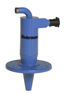
Cyclones are normally used when a maximum pre-separation of collected material from the transportation airflow is required. Cyclones are normally located on silos, tanks, containers etc. suitable to store the collected material and thereby function as a deead chamber under the cyclone. Normally, a filter stage shall be installed between the cyclone and the vacuum power unit
