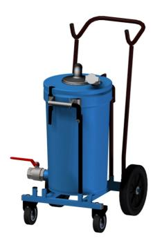
Mobile pre-separator for collecting and recycling of oil, cutting fluid, coolant, water and other non-flammable liquids. Perfect formachining and process industries, drilling, milling and turning. A float ball automatically shut off the suction flow when the container is full. The mobile pre-separator is equipped with a tippable container for easy discharge of collected liquids. The inlet and outlet diameter is 51 mm (2 in) for coupler (43930101 and 43930102).
