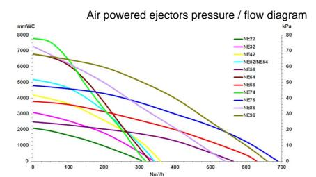
Air Powered ejectors
