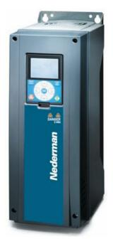
Frequency control to maintain a constant system pressure. Nederman Fan Inverter is a frequency controller that is preprogrammed with an extraction fan application for Nederman fans. It is equipped with a pressure sensor and a PID controller that can maintain a constant negative pressure in an extraction system.
