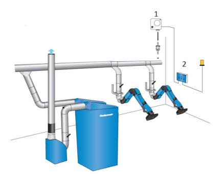
Airflow alarm and pressure switch mounted
