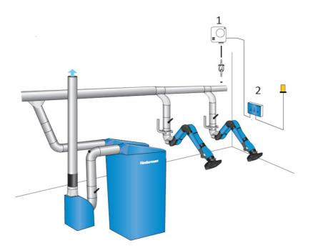
Airflow alarm and pressure switch mounted
